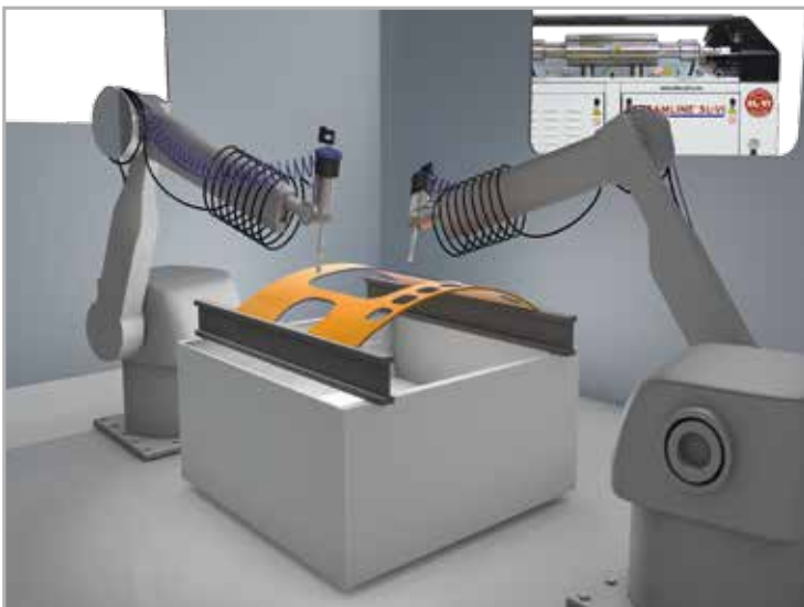
3D-Cutting Box with high pressure pump STREAMLINE SL-VI 100 PLUS
